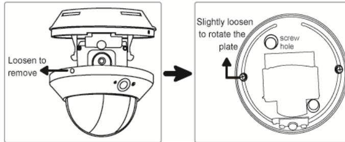
Step 3: Mark the locations of the two screw holes on the ceiling or wall, and drill a hole for each on the ceiling or wall. The distance between your camera and the location you want to monitor should be 3 ~ 4 meters.
