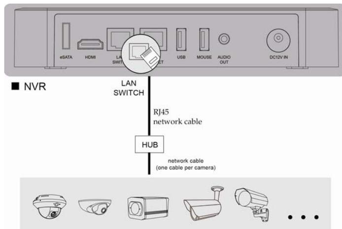
Step1: Connect PC to the HUB connected to your camera(s) with RJ45 network cable.
