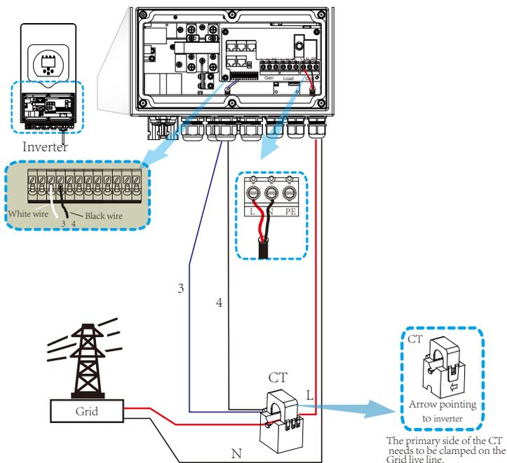
**\*Note:** when the reading of the load power on the LCD is not correct, please reverse the CT arrow.
