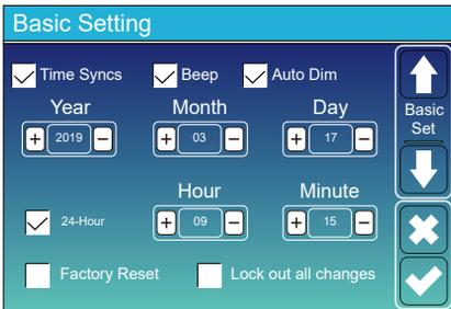
**Factory Reset:** Reset all parameters of the inverter.
