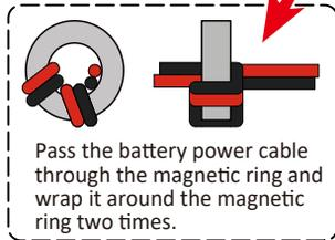
Pass the battery power cable through the magnetic ring and wrap it around the magnetic ring two times.
