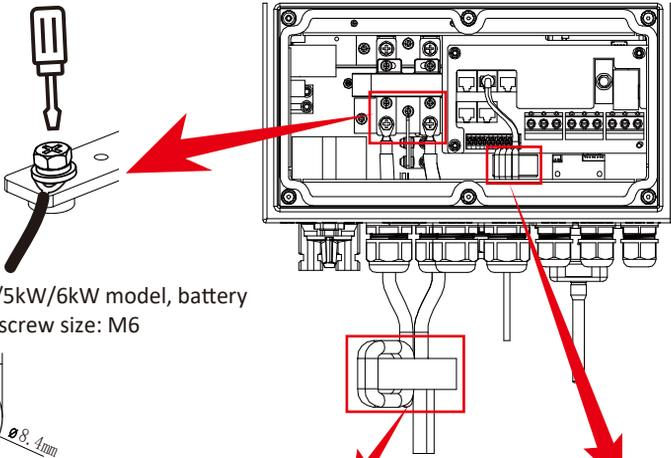
For 3.6kW/5kW/6kW model, battery connector screw size: M6
