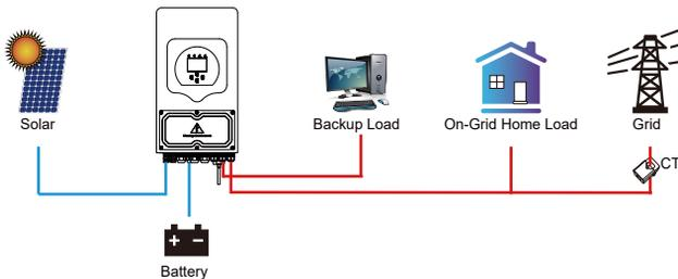
**Solar Sell:** “Solar sell” is for Zero export to load or Zero export to CT: when this item is active, the surplus energy can be sold back to grid. When it is active, PV Power source priority usage is as follows: load consumption and charge battery and feed into grid.
