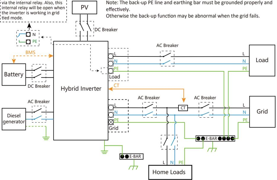
This diagram is an example for application that Neutral connects together with PE in distribution box.
