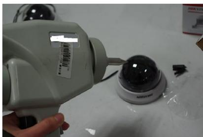
Test device for electrostatic discharge anti-interference
