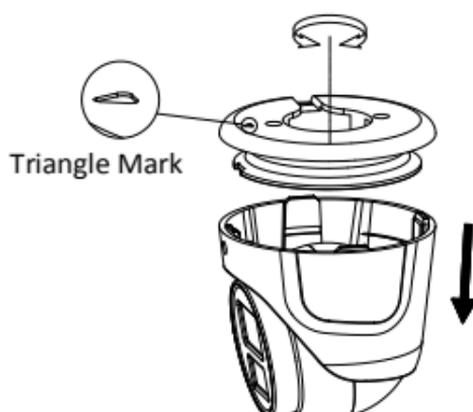
Figure 2-2 Disassemble the Camera
