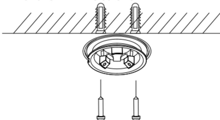
Figure 2-4 Install the Mounting Base to Cement Ceiling
