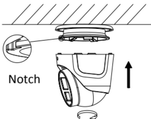
Figure 2-5 Align the screw hole to the Notch
