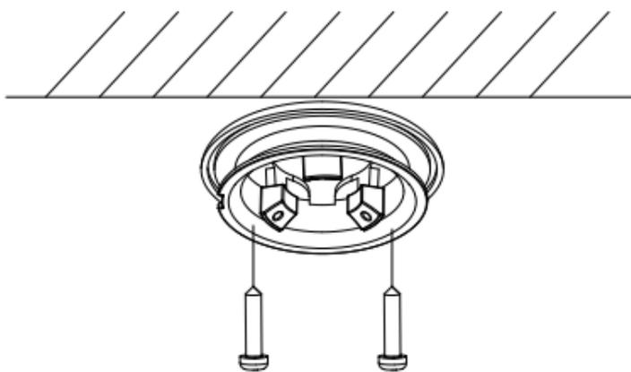
Figure 2-3 Install the Mounting Base to Wooden Ceiling
