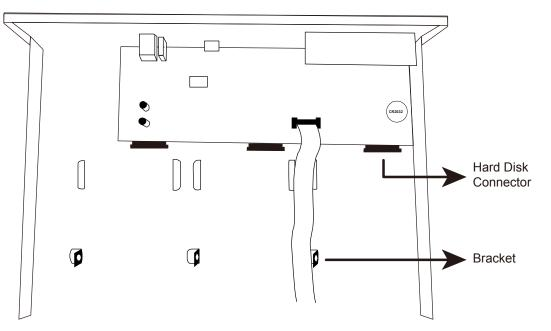
Step2: Get a compatible hard disk. With the PCB side facing down, insert the hard disk to one of the hard disk connector.
