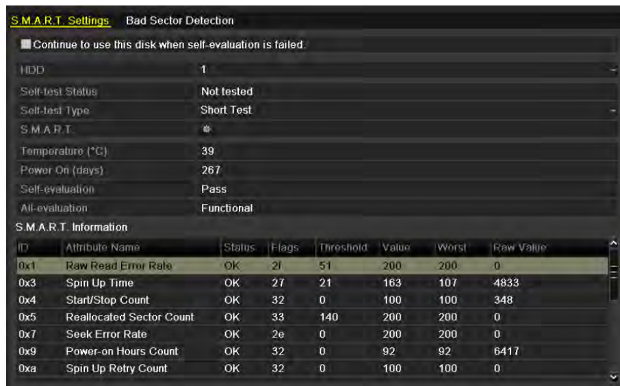
Figure 10. 22 S.M.A.R.T Settings Interface
