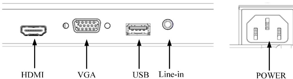
Figure 1-2 Interfaces on the Rear Panel
