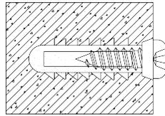
**Figure 2-2 Insert Plastic Sleeve**
