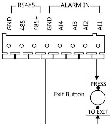
Figure 4-9 Exit Button Wiring for DS-KD3002-VM
