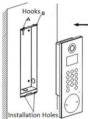
Figure 5-4 Install the Door Station
