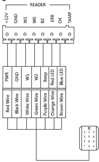
Figure 4-11 External Card Reader Wiring
