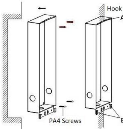
Figure 5-9 Insert the Gang Box into the Wall
