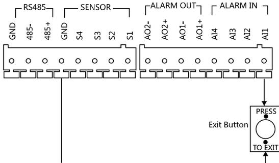
Figure 4-7 Exit Button Wiring for DS-KD8102-V/DS-KD8002-VM (1)
