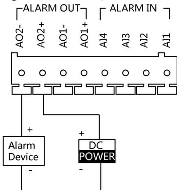
Figure 4-15 Alarm Device Output Wiring for DS-KD8102-V/DS-KD8002-VM
