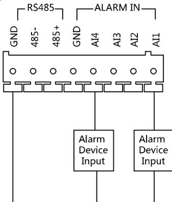
Figure 4-14 Alarm Device Input Wiring for DS-KD3002-VM
