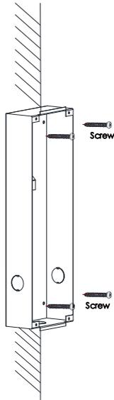
Figure 5-13 Insert the Gang Box into the Wall
