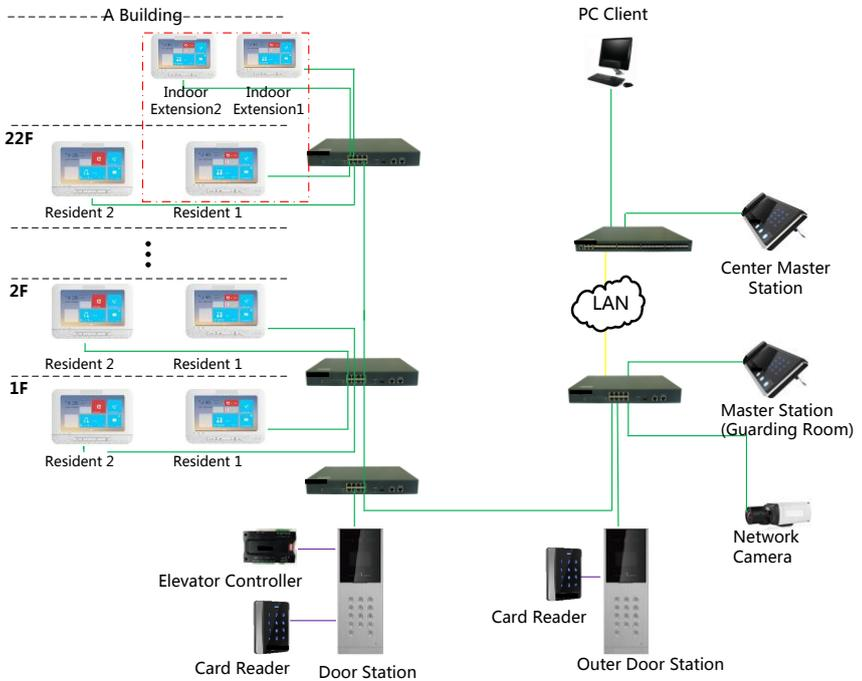
Figure 3-1 Typical Application of Door Station
