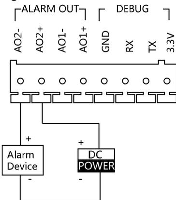
Figure 4-16 Alarm Device Output Wiring for DS-KD3002-VM
