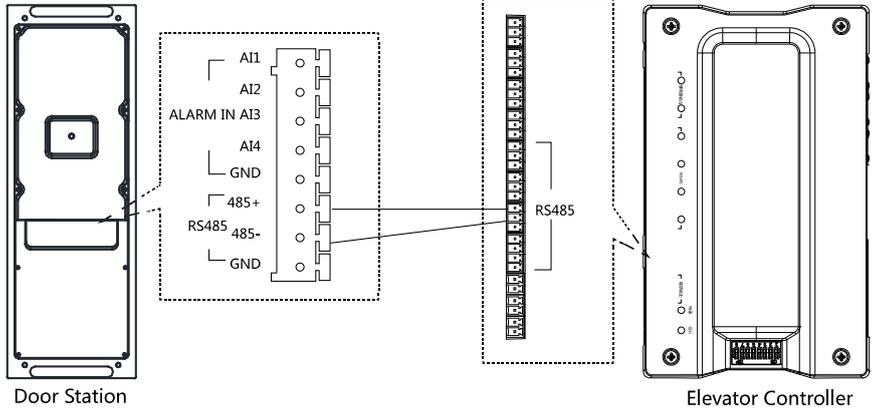
Figure 4-12 External Elevator Controller Wiring
