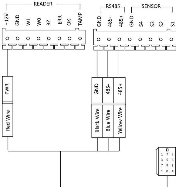
Figure 4-10 RS-485 Card Reader Wiring
