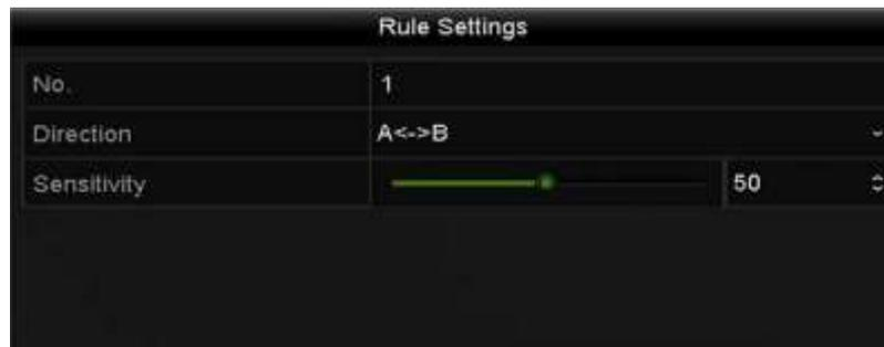
Figure 10-6 Set Line Crossing Detection Rules
