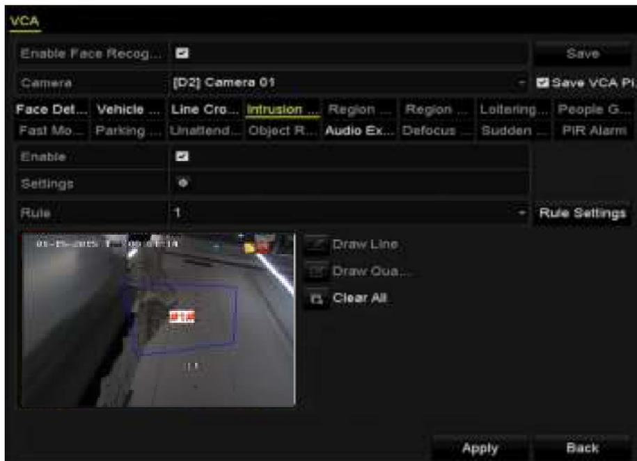
Figure 10-9 Draw Area for Intrusion Detection
