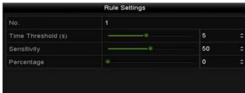
Figure 10-8 Set Intrusion Crossing Detection Rules
