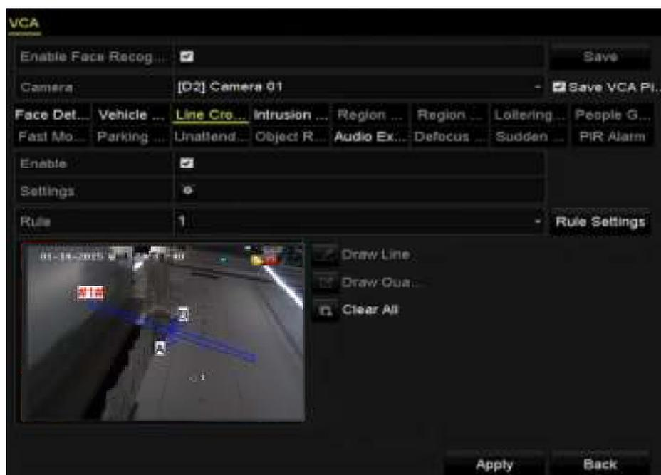
Figure 10-7 Draw Line for Line Crossing Detection
