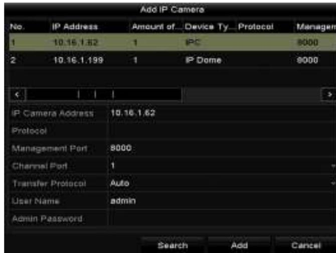
Figure 2-28 Quick Adding IP Camera Interface
