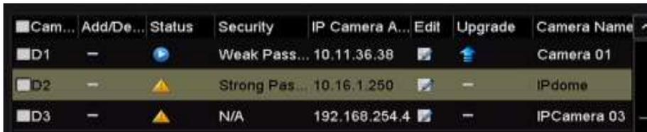
Figure 2-32 Security Level of IP Camera's Password
