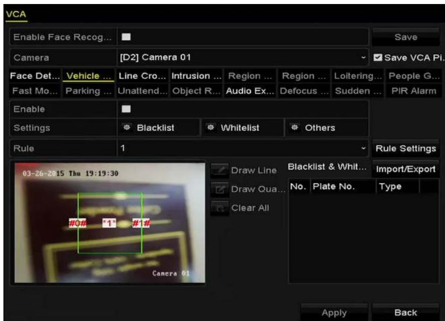
Figure 10-4 Set Vehicle Detection
