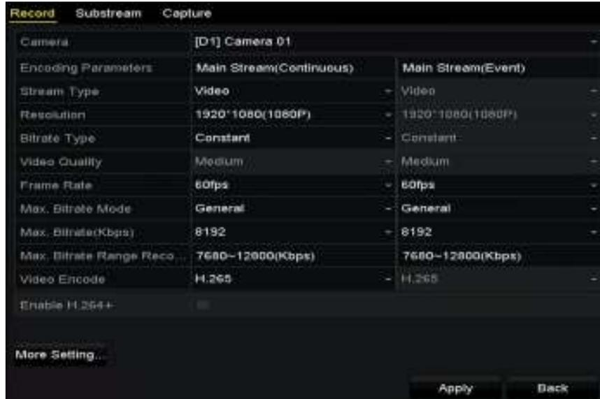
Figure 5-3 Recording Parameters
