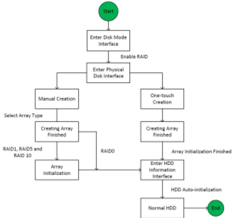
Figure 13-1 RAID Working Flow
