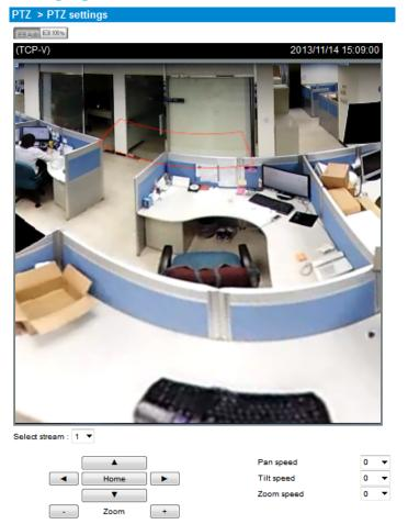
In this window, functional items related to the preset positions have been cancelled. This window is now used for changing the field of view when the Local dewarp is applied to a video stream.
