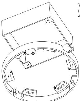
You may also use the diagonal holes on the mounting plate, marked as A, B, or C, to install the camera to a U.S. standard 4 in. junction box.
