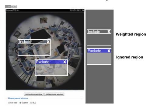
■ BLC (Back Light Compensation): This option will automatically add a "weighted region" in the middle of the window and give the necessary light compensation.
