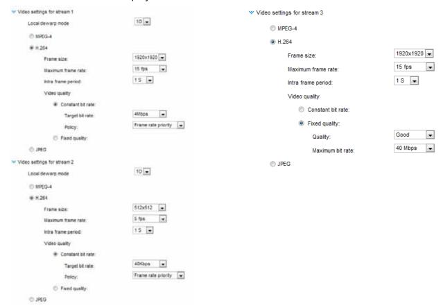
This Network Camera offers real-time H.264, MPEG-4 and MJPEG compression standards (Triple Codec) for real-time viewing.
