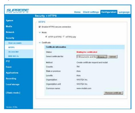
11. When the certifice file is successfully loaded, its status will be stated as **Active**. Note that a certificate must have been created and installed before you can click on the "**Save**" button for the configuration to take effect.
