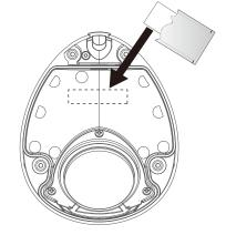
Attach the dome cover to camera. Secure the dome screws with the supplied screwdriver. Finally, make sure all parts of the camera are securely installed.
