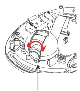
Tighten the lens lock screw.
