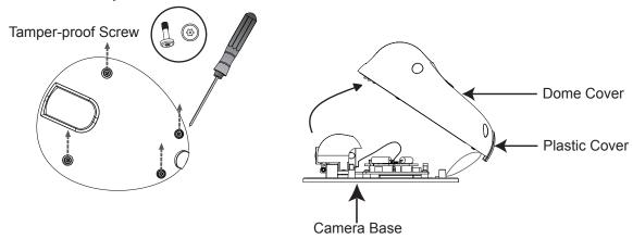
Then, follow the steps below to install the camera to either the ceiling or the wall:
